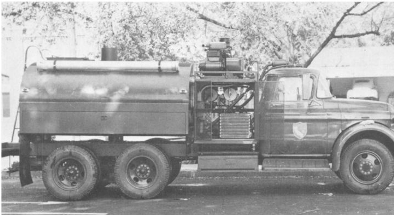
FIGURE 31. 1961 model fish hauling truck; 2,000-gallon water capacity; V-6 engine under the hood; carrying capacity 3,000 pounds of 6- to 10-inch trout. Gasoline powered generators develop power for operating water circulating pumps and refrigeration units. Aeration of water is by a combination of venturi aspirator and overhead spray. Photograph by Williams.
