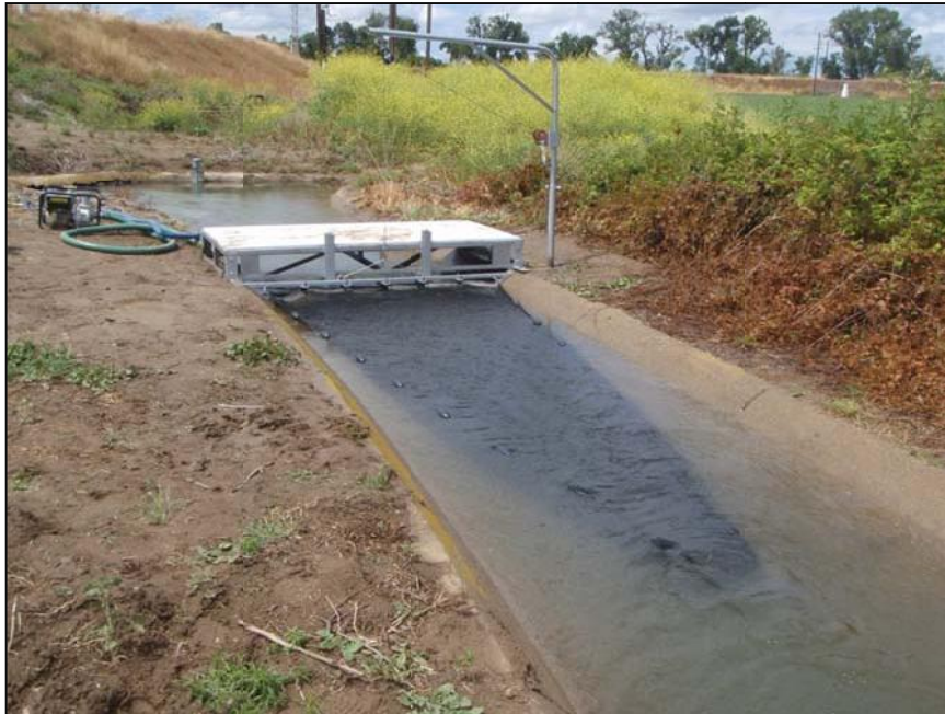
Figure 6. Fyke apparatus, fyke net, and sampling platform used to sample for fish entrainment in the Oji canal.
