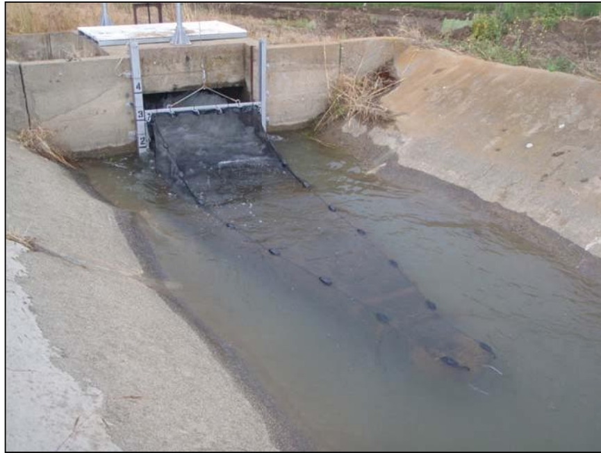
Figure 7. Fyke apparatus, fyke net, and sampling platform used to sample for fish entrainment in the Windswept canal.
